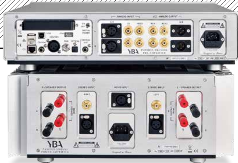
ABOVE: Novelties are revealed to the rear: preamp [top] packs an Apple AirPlay module to the left, below which are network and I 2 S digital connections on RJ45 sockets. The 'extra' mono XLR input on the power amp is for bridged operation
